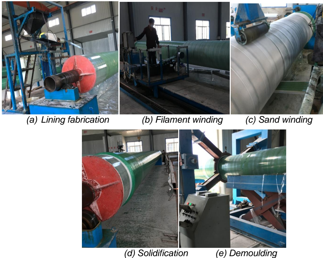
Fig.3 - Fabrication process of the filament-wound pipe
