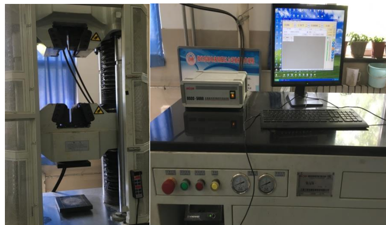
Fig. 5 - WAW-1000 universal testing machine
