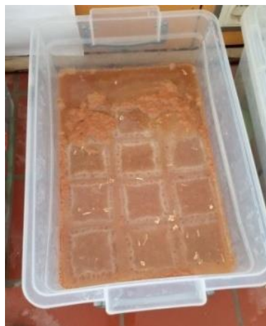
Fig. 5 - Cubic specimens 50 mm immersed in HCl 5% solution.
