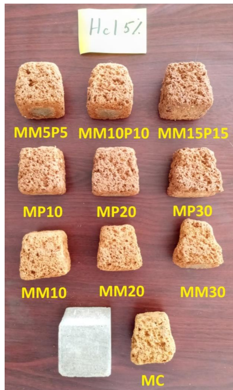
Fig. 14 - The ten mortars after 15 weeks exposed to HCl 5%.
