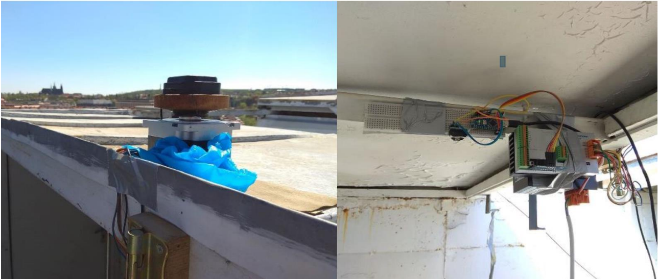
Fig. 4 – Device for automatic rotation - Antenna and stepper motor (left) Control unit of stepper motor, Arduino Nano and real time clock module (right)
