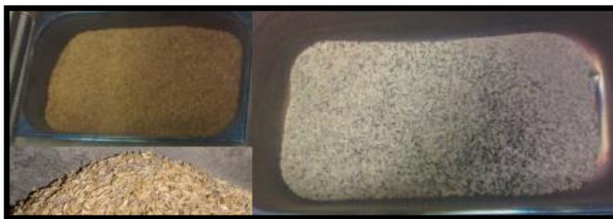
Fig. 1 – Rice husks before and after calcining.
