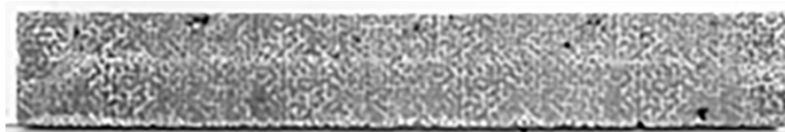
Fig. 4 – Speckled surface of the tested specimen
