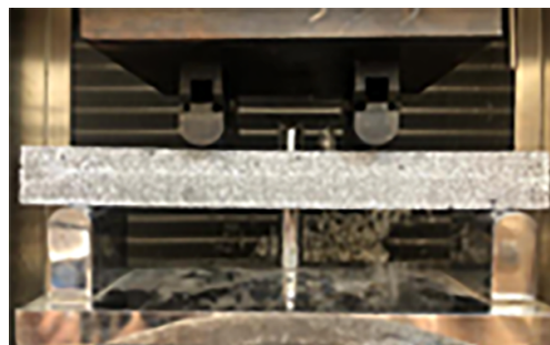
Fig. 5 – Four-point bending test
