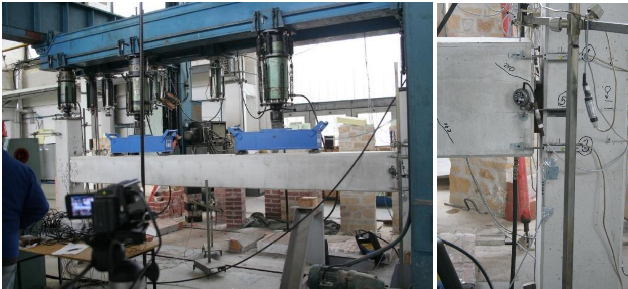
Fig. 5 – Test configuration (on the left) and the distribution of LVDT sensors at joint B (on the right)
