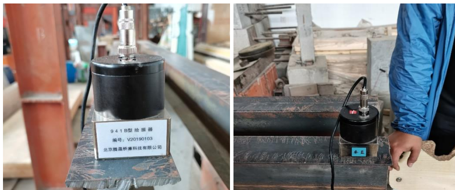
(a) Sensors at the girder end
