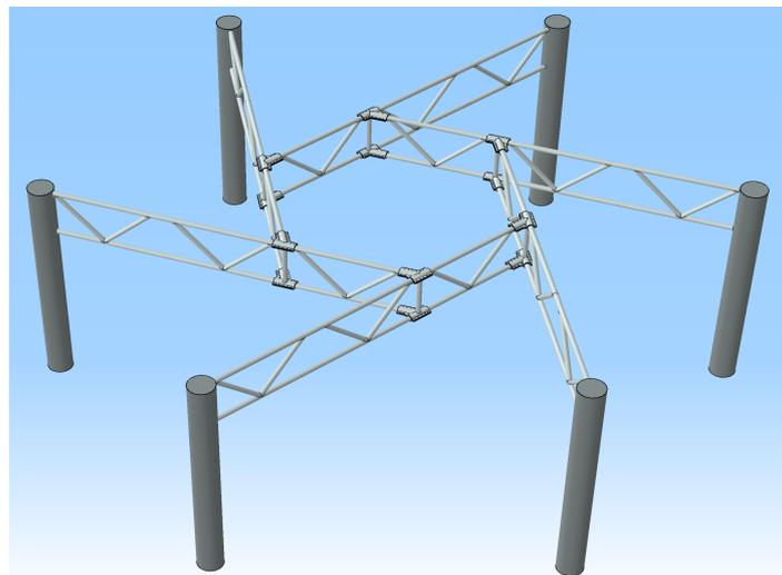
*Fig. 6. - A fan of double-layer of reciprocal frame*
