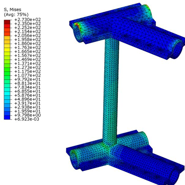
Fig. 13 - Stress nephogram of the prefabricated connector/Pa
