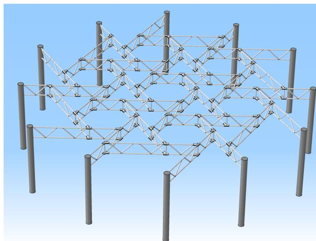
Fig. 28 - Double-layer reciprocal frame
