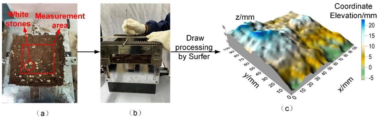
Fig.3- Extraction process of the 3D topography of the shear surface: (a) the actual shear surface after shearing; (b) the measurement diagram of the shear surface; (c) the 3D topography map of the shear surface
