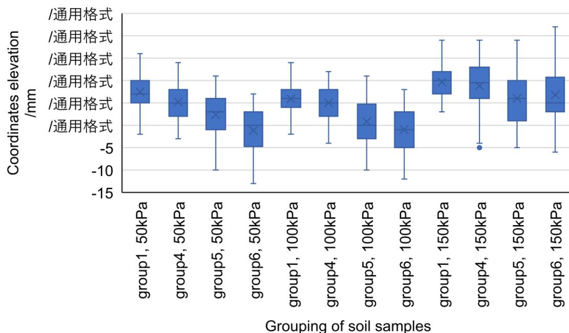
Fig.7- Elevation statistics of shear failure surface coordinates
