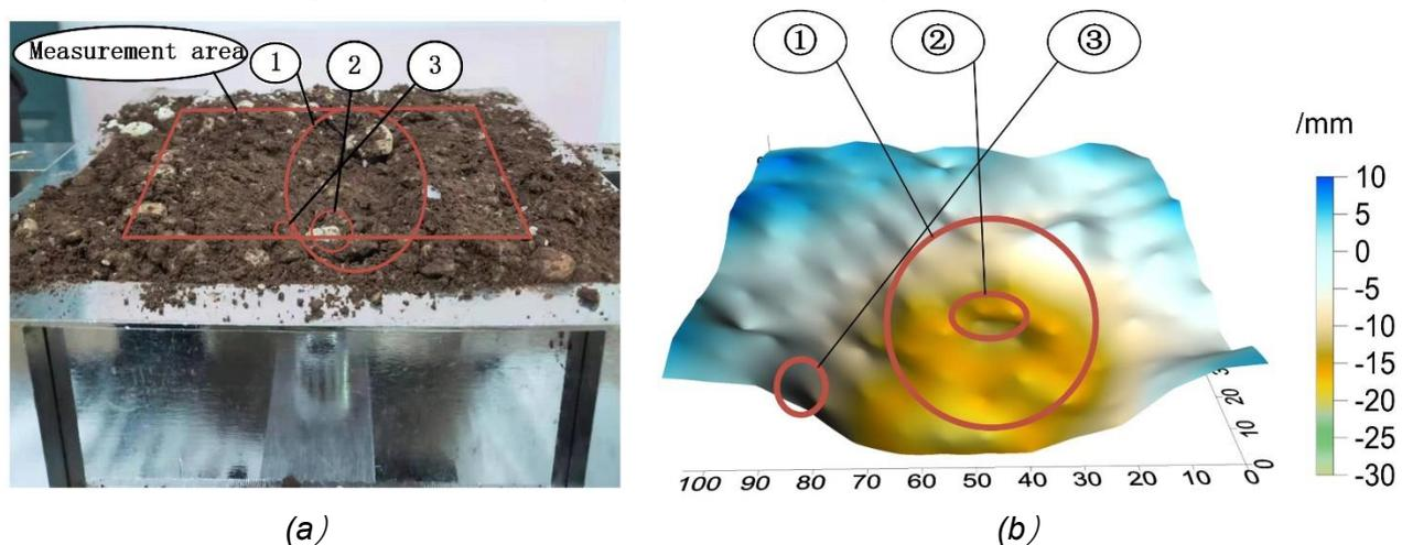
Fig.5- Comparison between the shear surface 3D topography map and the actual shear surface:
