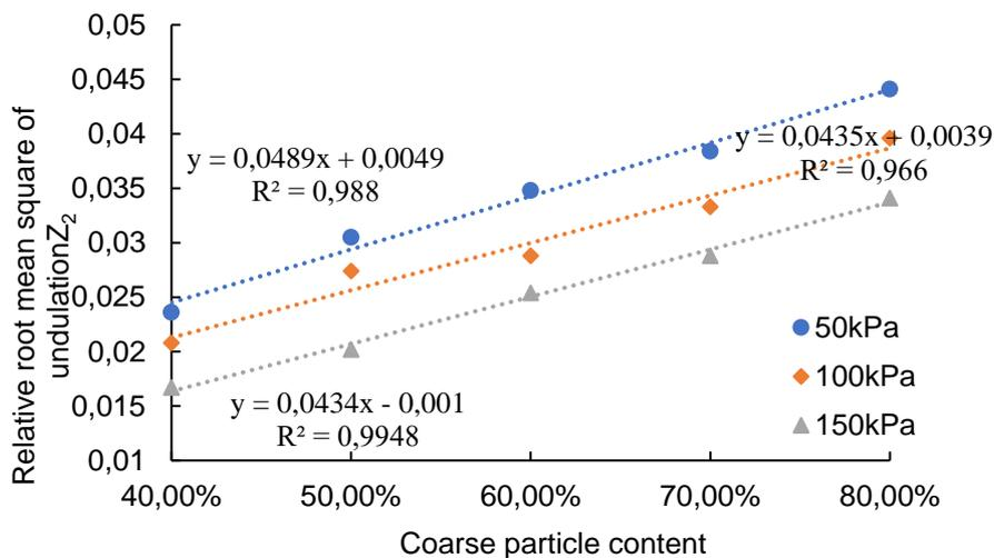
Fig. 14- Relationship between shear surface roughness and coarse grain content of slip zone soil
