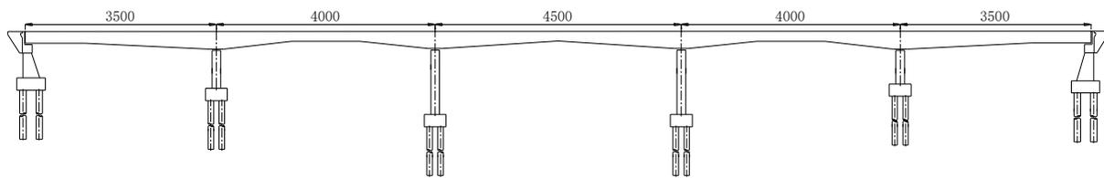
*Fig.1 - Bridge Elevation Layout (Unit: cm)*
