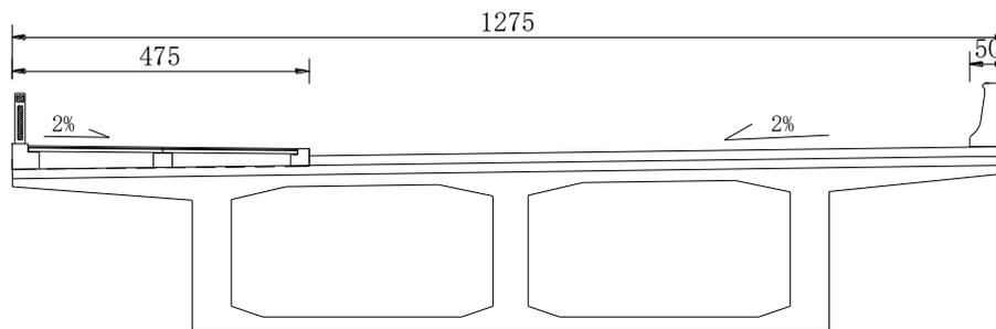
*Fig.2 - Bridge cross section (Unit: cm)*
