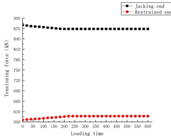
Fig.12 - Relationship curve between load holding time and tension of F3e steel
