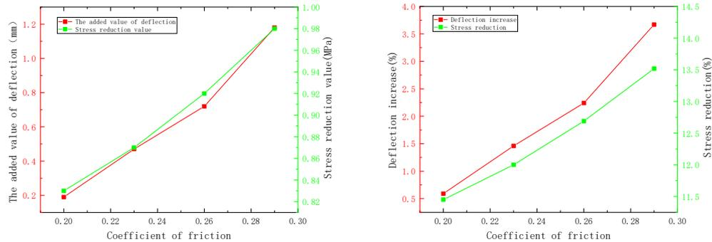
Fig. 14 - Influence of friction coefficient alone on deflection and stress of main beam
