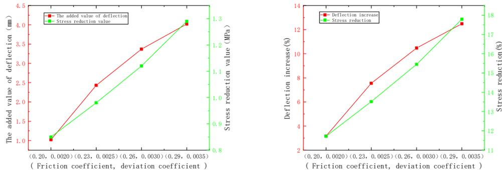
Fig. 16 - Coupling changes of friction coefficient and deviation coefficient on deflection and stress of main beam Influence diagram
