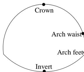
Fig. 4 - Key positions of the tunnel
