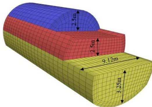
Fig. 3 - Schematic diagram of the construction method
