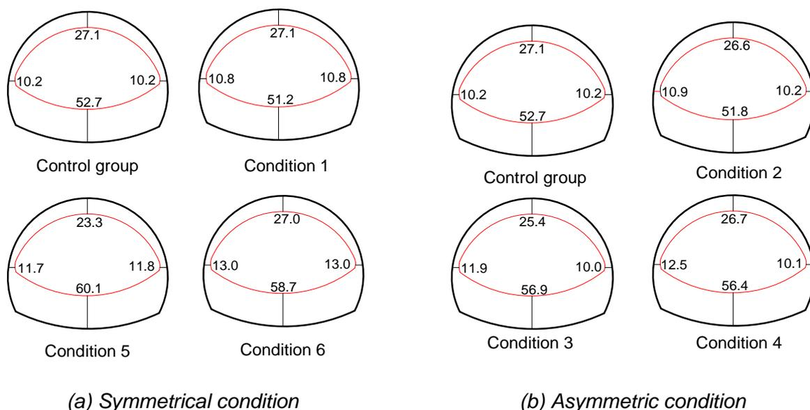
Fig. 6 - Distribution law of tunnel deformation under different arrangements of softening positions /mm
