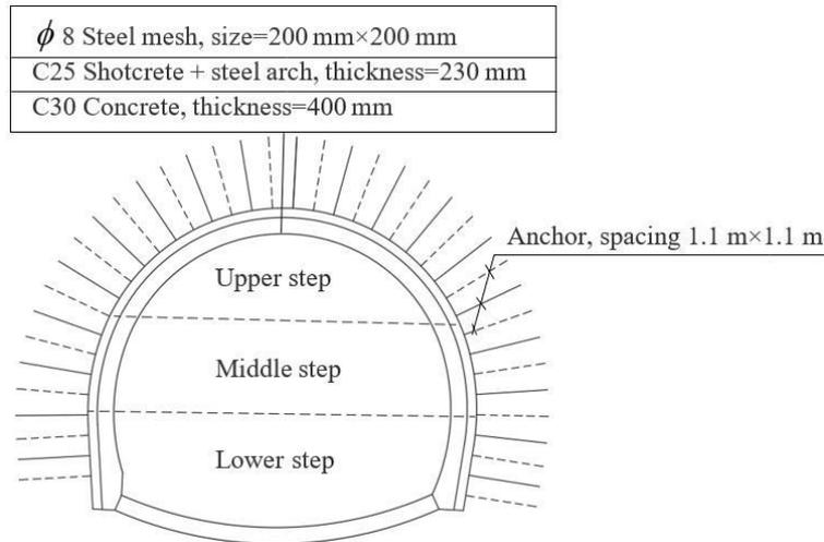
Fig. 1 - Schematic diagram of the tunnel section
