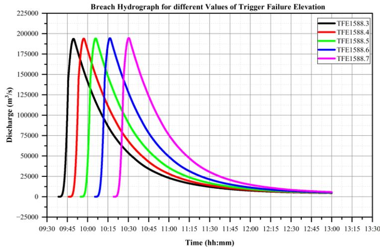
Fig. 10 - Breach hydrograph for different values of trigger failure elevation
