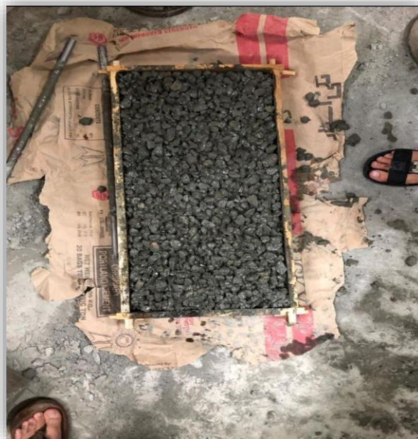
Fig. 3 – Slab placed in its Custom Wooden Mould
