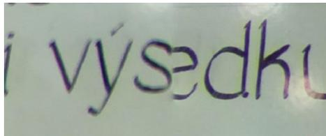
Fig. 6 – Bad stitching of images from camera rig
