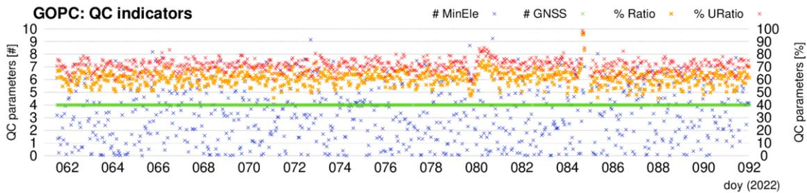
Fig. 6 - GOPC station parameters (GPS, GLO, BDS, GALILEO)
