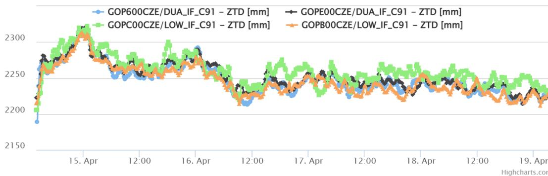
Fig. 9 - An assessment of the tropospheric characteristics of the stations situated at the Pecny Observatory.
