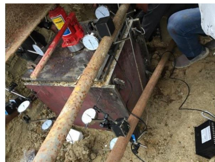
(b) On-site dial indicator installation
