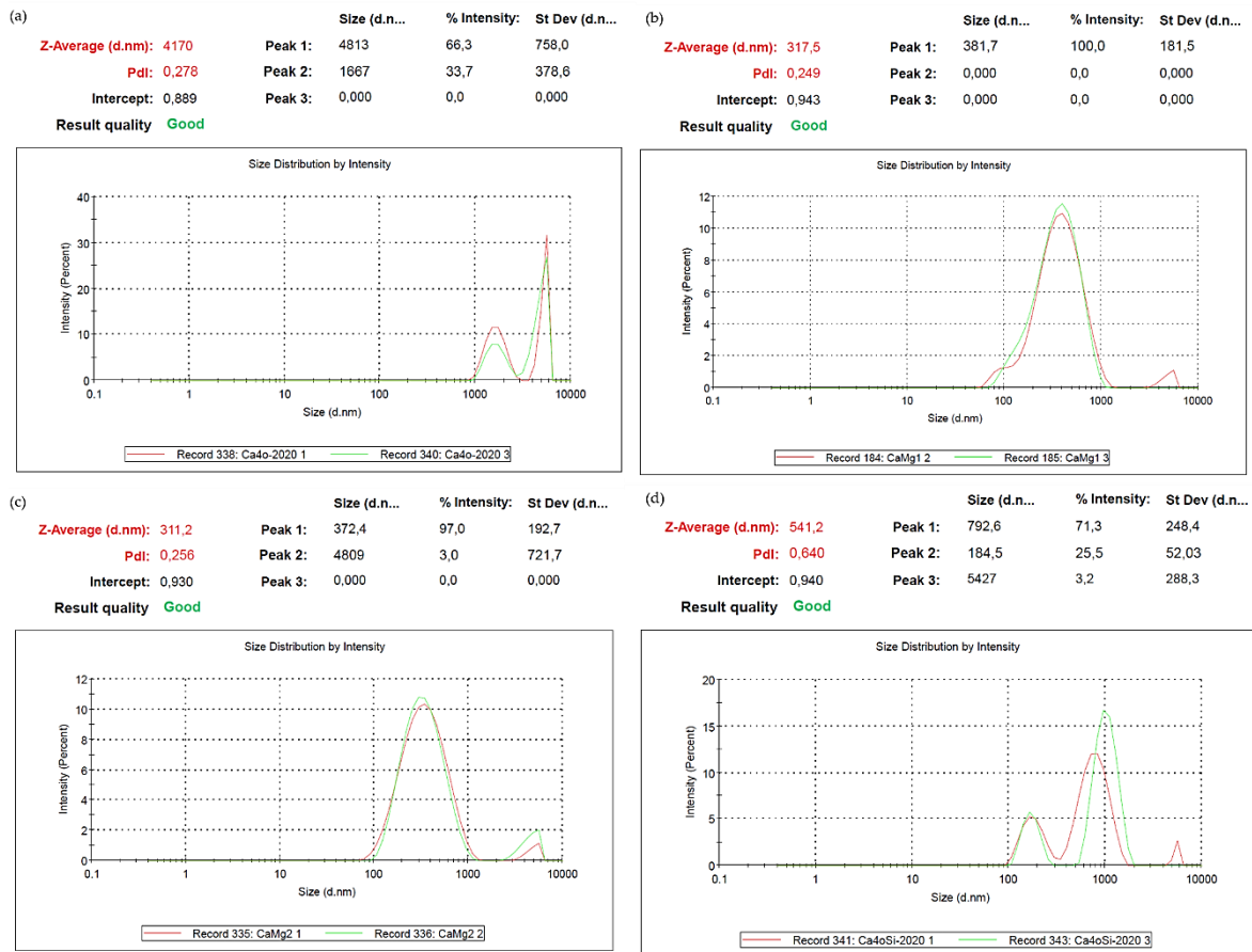
Fig. 1 - Ca(OH) 2 particle size in nanolime suspensions was measured by the dynamic light scattering (DLS) method. The Malvern Zetasizer ZS device was used for the measurement: a) CaMg1; b) CaMg1; c) CaMg2; d) Ca4O-Si.
