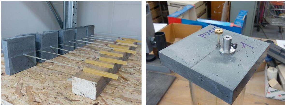
*Fig. 1 – Specimens preparation for the pull-out test.*
