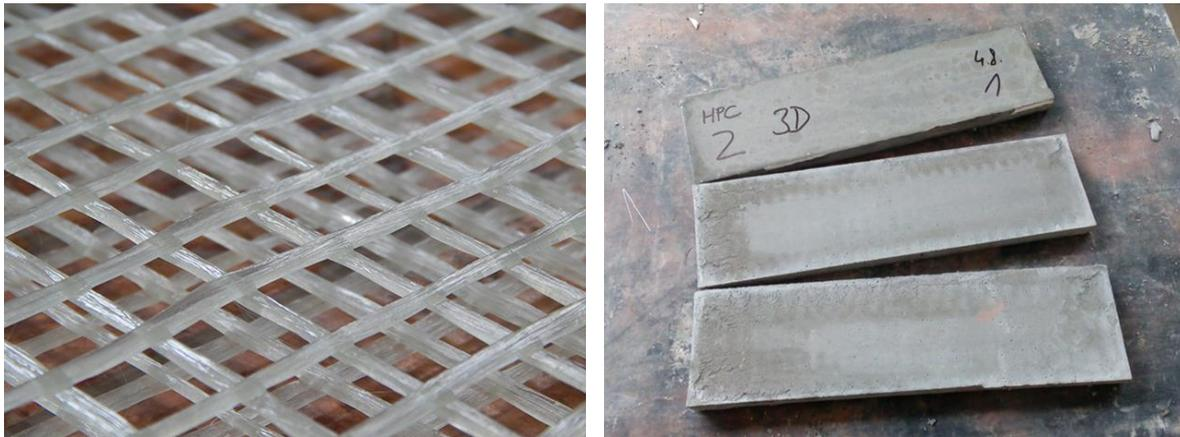
*Fig. 2 – Specimens preparation for the four-point bending test.*
