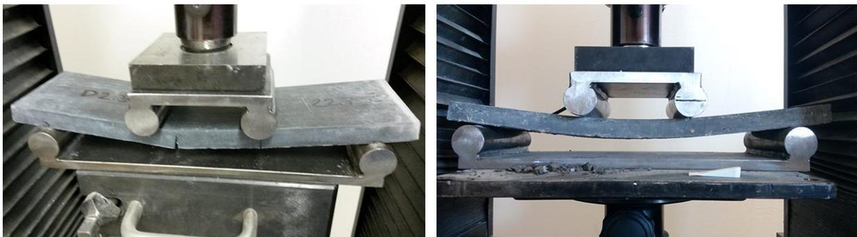
Fig. 7 – Typical crack development of 2x5 reinforcement with smooth surface on the left and 4x10 reinforcement treated with fine-grained silica sand on the right side.
