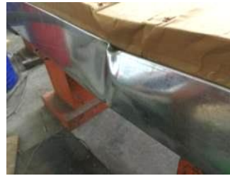
(b) – Buckling failure of steel beam-A
