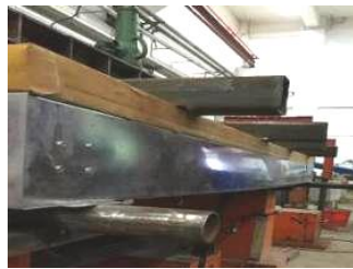
(e) – Deformation of steel beam-C
