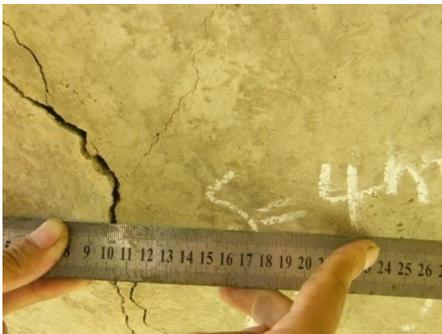
(c) longitudinal bottom crack of second span (L=0.7m δ=4mm)
