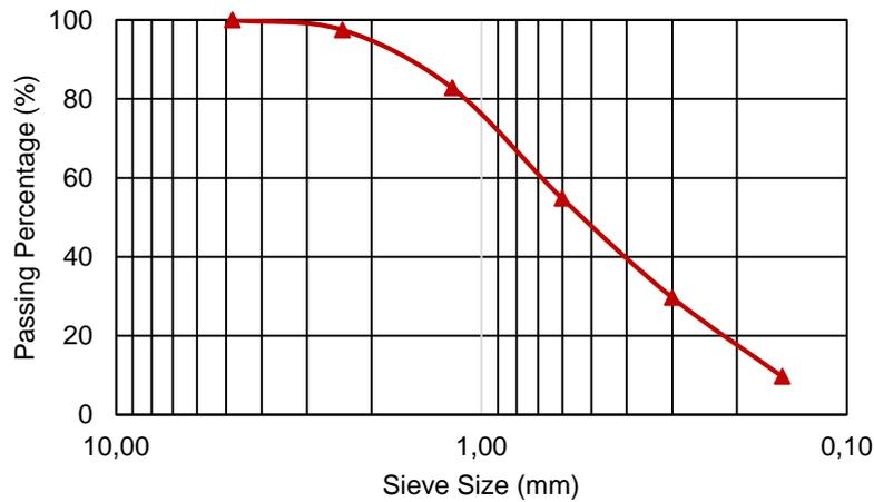
Fig. 1 - Gradation of fine aggregate
