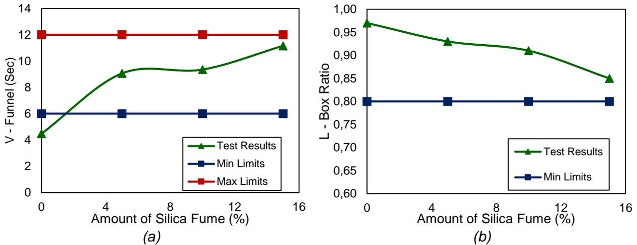
Fig. 3 – (a) V-funnel; (b) L - Box ratio on varying silica fume on SFCC
