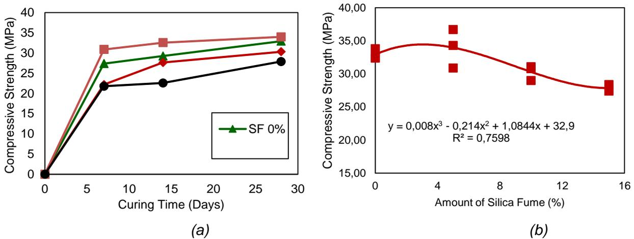
Fig. 5 – Effect of varying silica fume and curing age on Compressive strength SFCC in different curing time
