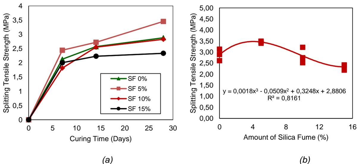
Fig. 6 – Effect of varying silica fume on tensile strength of SFCC in different curing time
