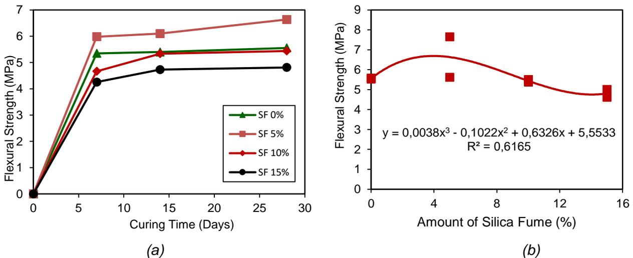
Fig. 7 – Effect of varying silica fume on flexural strength of SFCC in different curing time
