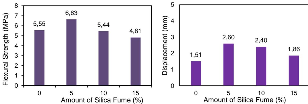
Fig. 8 – Effect of varying silica fume on flexural strength of SFCC in different curing time
