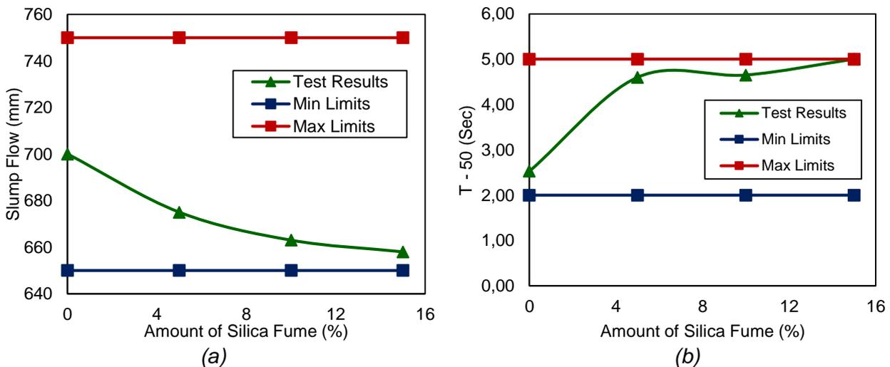
Fig. 4 – (a) Slump flow; (b) T50 result on varying silica fume on SFCC
