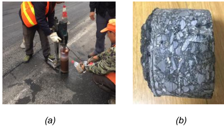
Fig.12 - Drilling core sample and the core sample
