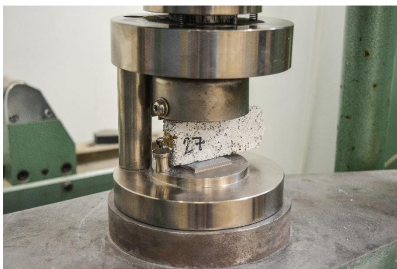
Fig. 3 – The compression test of specimens: The auxiliary loading device with two auxiliary platens was placed in the hydraulic testing machine with selected specimens prepared for the test
