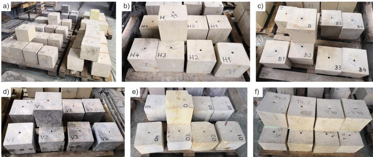
Fig. 1 – a) Stone a mortar test specimens, b) Coarse-grained sandstone test specimens (Hořice), c) Fine-grained sandstone (Božanov), d) Limestone test specimens, e) Marlstone test specimens, f) Mortar test specimens
