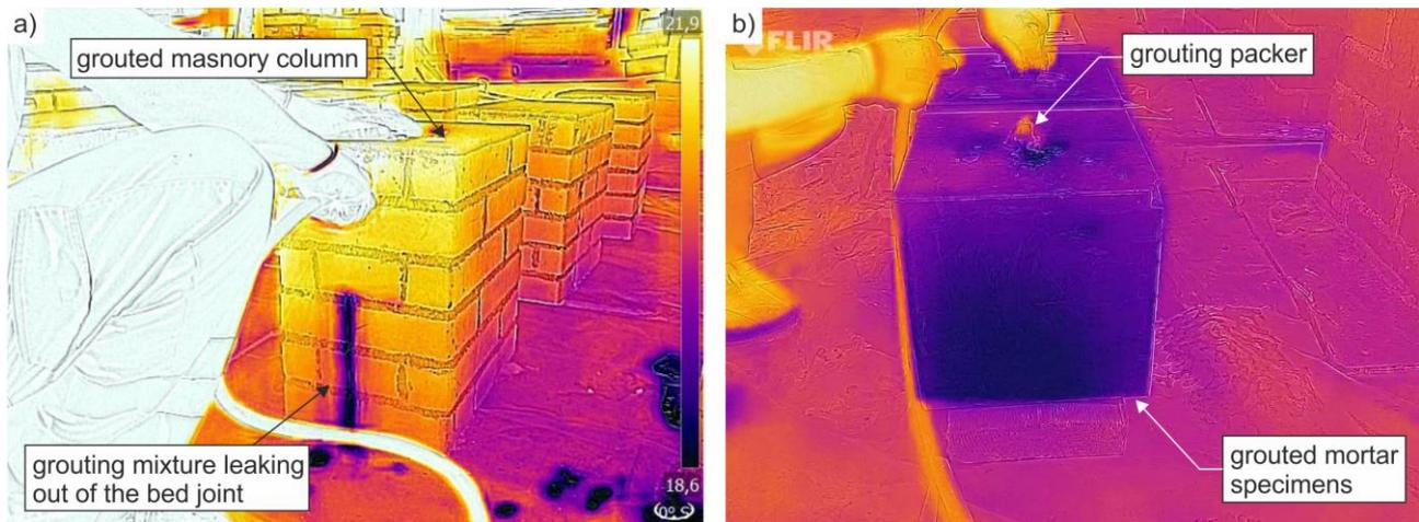
Fig. 4 – a) Thermovision image captured during grouting brick masonry test specimen with hydraulic lime based grouting mixture with nanosuspension labelled BV7, b) Thermovision image captured during grouting mortar test specimen with hydraulic lime based grouting mixture labelled BV3
