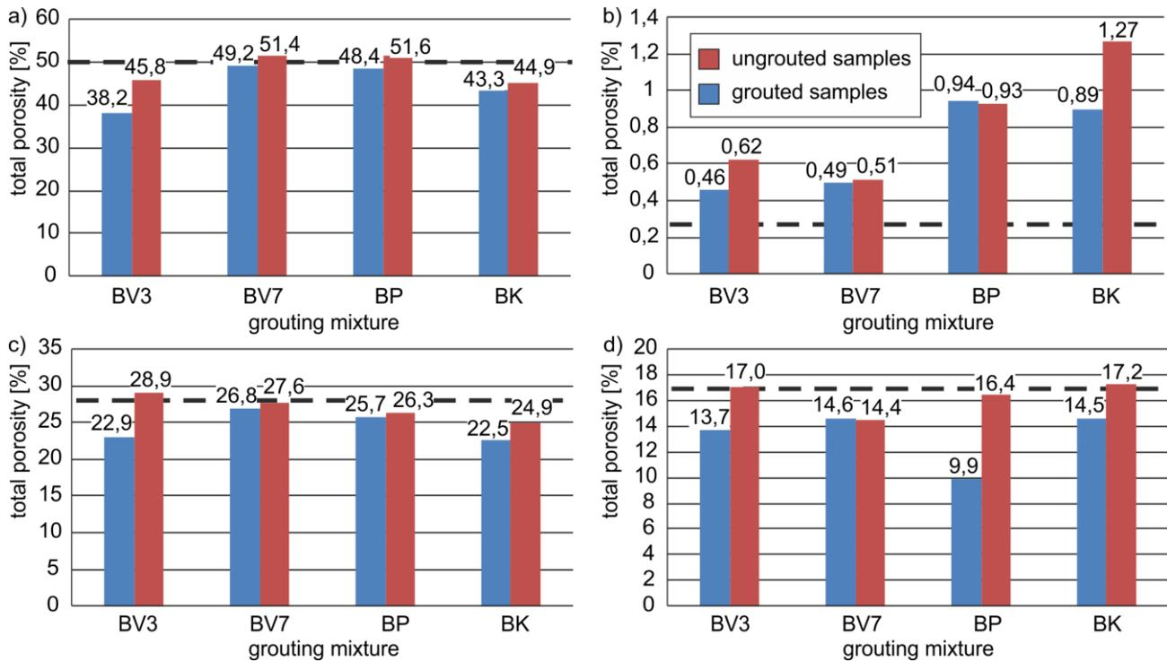
Fig. 3 – Comparison of total porosity of selected materials before and after grouting, a) Marlstone, b) Limestone, c) Coarse-grained sandstone (Hořice), d) Fine-grained sandstone (Božanov)
