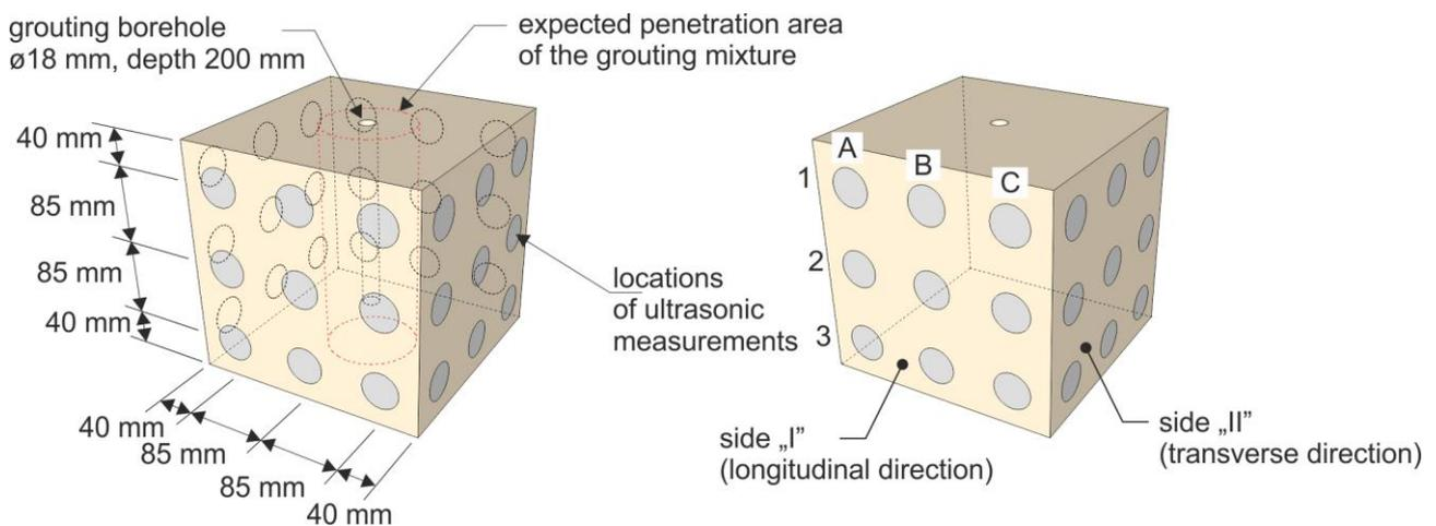
Fig. 5 – Ultrasonic testing scheme
