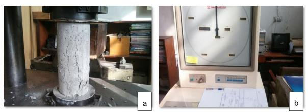
Fig. 3 – (a) & (b) Compressive test of concrete cylinder
