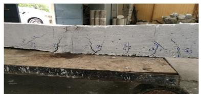
Fig. 8 – Crack pattern in 40% PCA specimen DOI 10.14311/CEJ.2019.02.0021
