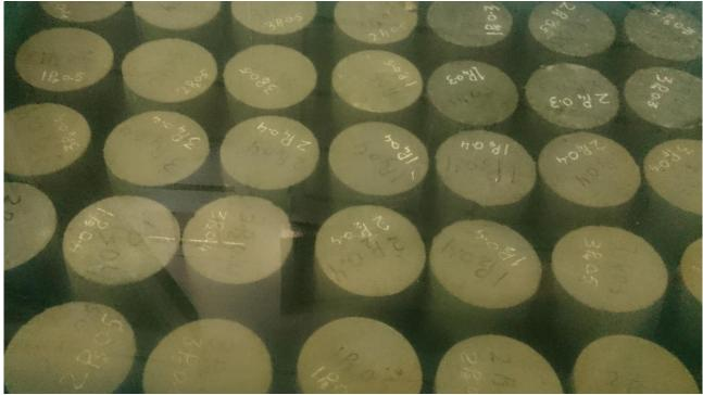
Fig. 2 – Curing stage of concrete cylinder
