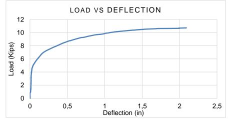
Fig. 7 – Average load vs. deflection curves for beams having W/C=0.3, PCA=40%
