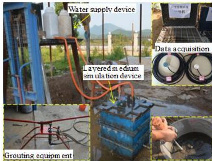
Fig. 8 – Picture of the experimental set-up
