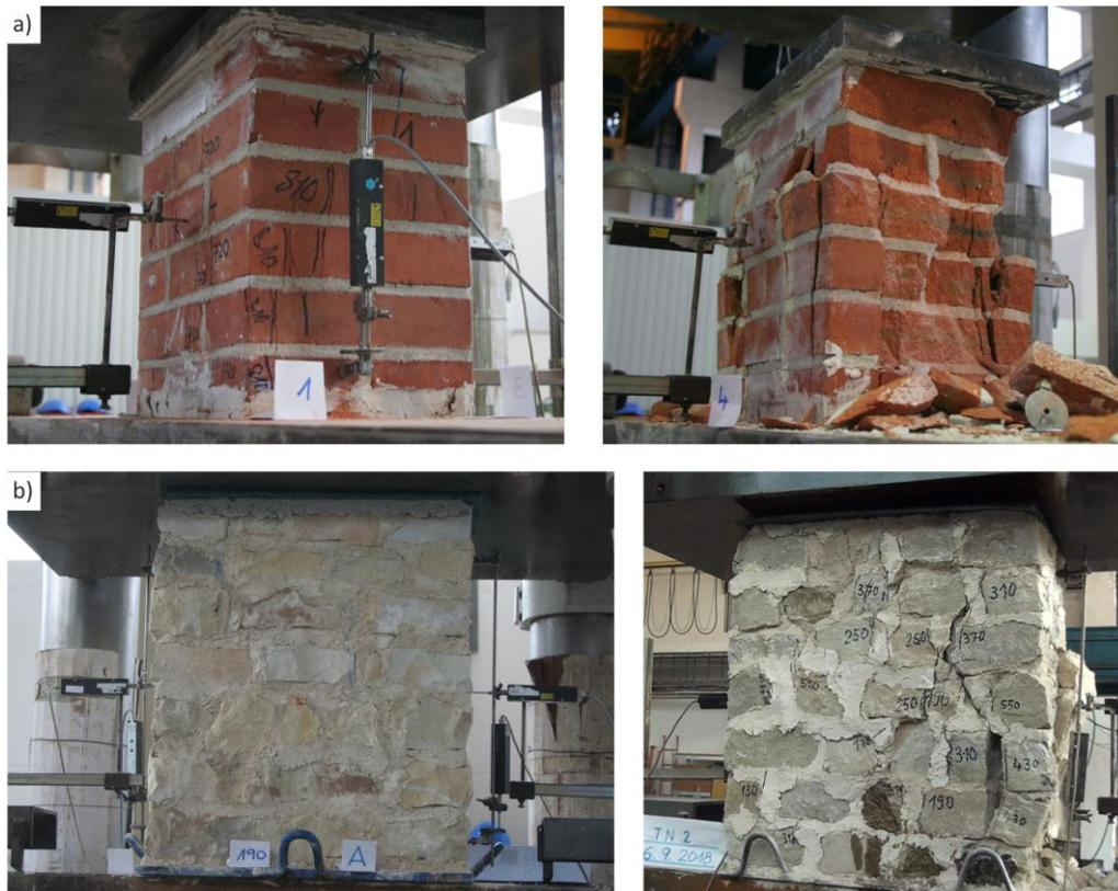
Fig. 2 - Experimental test pieces of brick (a) and stone (b) masonry during compressive tests
