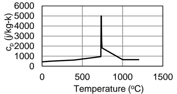
Fig. 7 - Variation of specific heat of steel with elevated temperatures [10]
