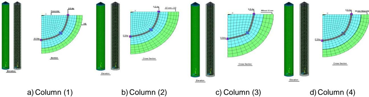
Fig. 23 - Finite element 3-D model of columns in ANSYS
