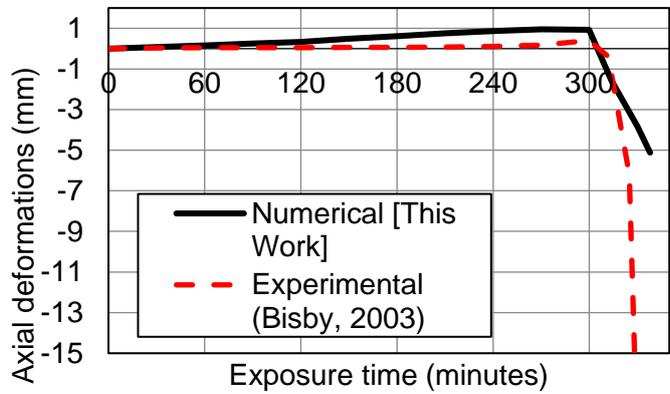
Fig. 31 - Column (2): Axial deformation of the column during fire exposure
