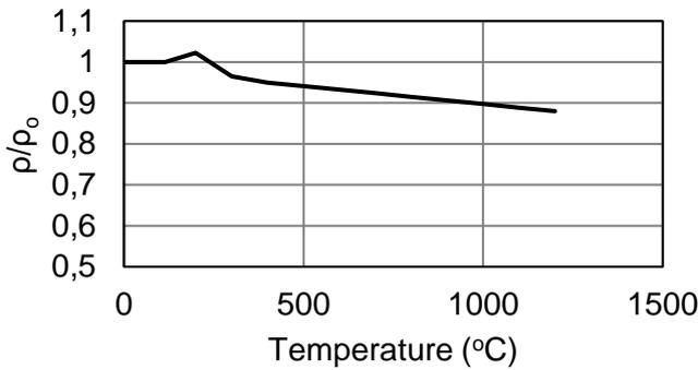
Fig. 1 - Variation of density of concrete with temperature [9]
