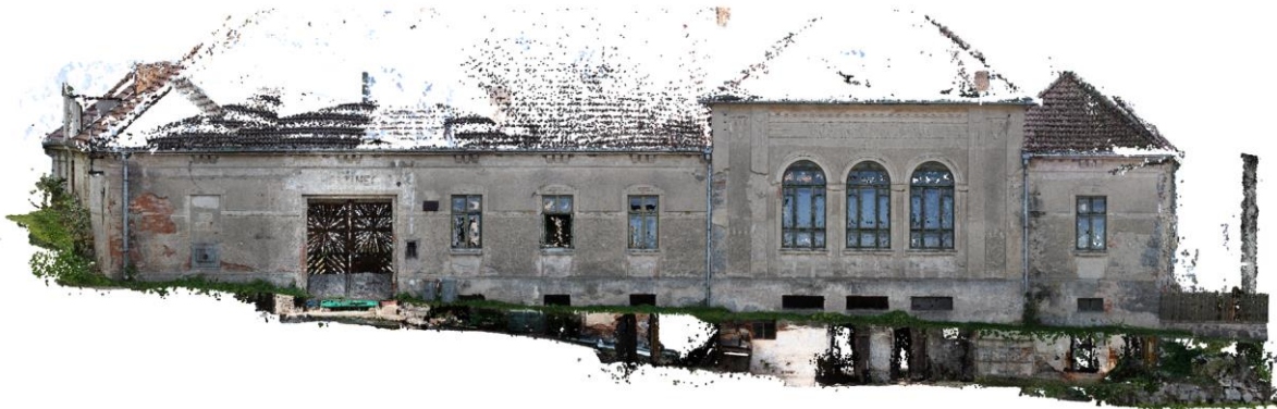
Fig. 9 - Example of the point cloud, front view, Kostelec nad Vltavou (Písek District, Czech Republic)
