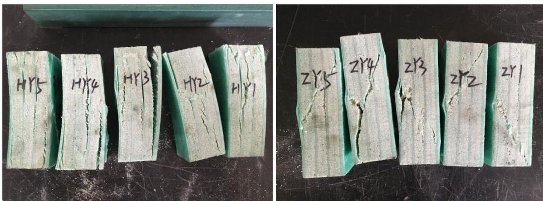
Fig. 8 - Ring and axial sample destruction form
