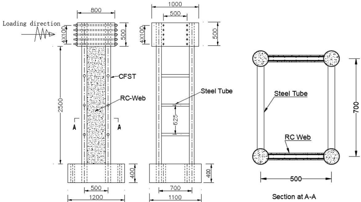
Fig. 1 - Details of CFST-RC Pier
