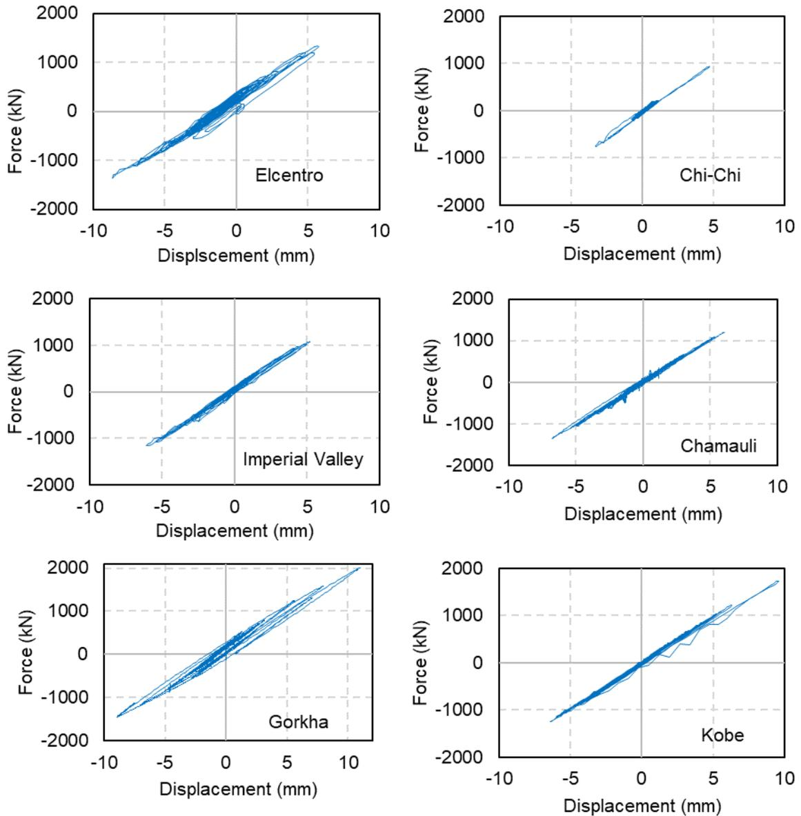
Fig. 10 - Force Displacement Hysteretic Curves
