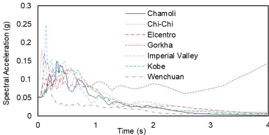
Fig. 5 - Scaled Pseudo-Acceleration Response Spectra (5% Damping)
