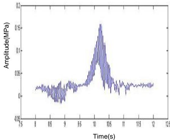
(b) Signal de-noised through the wavelet transform
