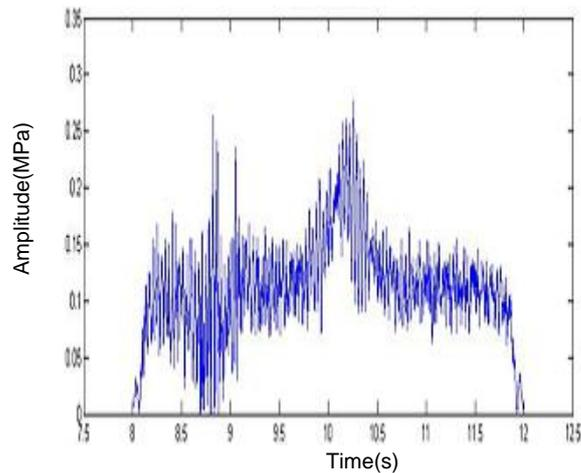
(b) Signal de-noised through frequency domain low-pass filtering
