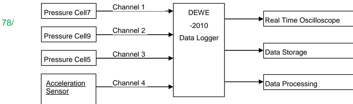
Fig.1 - Experimental setup
