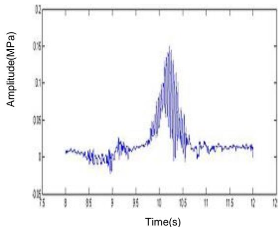
(b) Signal de-noised through spectrum subtraction
