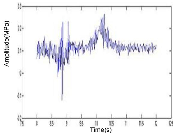
(b) De-noised signal through wavelet transform
