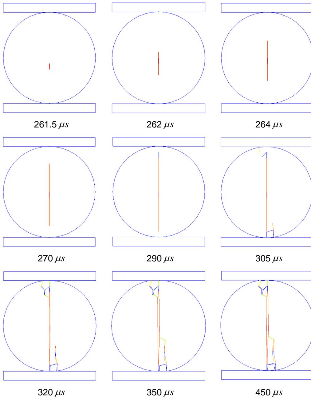
Fig.6 - Crack initiation and propagation of BTS test
