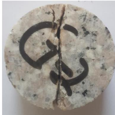
Fig.3 - Fracture pattern of BTS test
