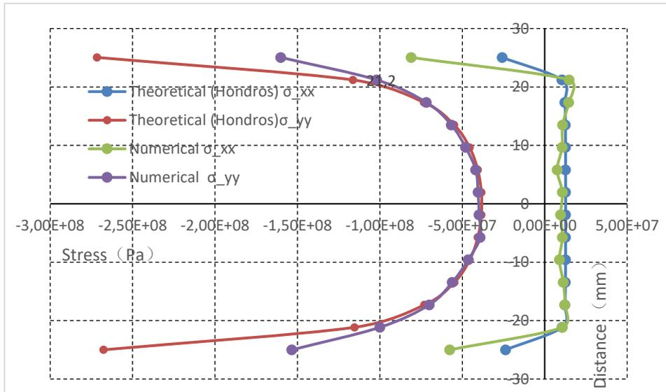
Fig.9 - Theoretical and numerical results of stresses distribution across loaded diameter for disc specimen
