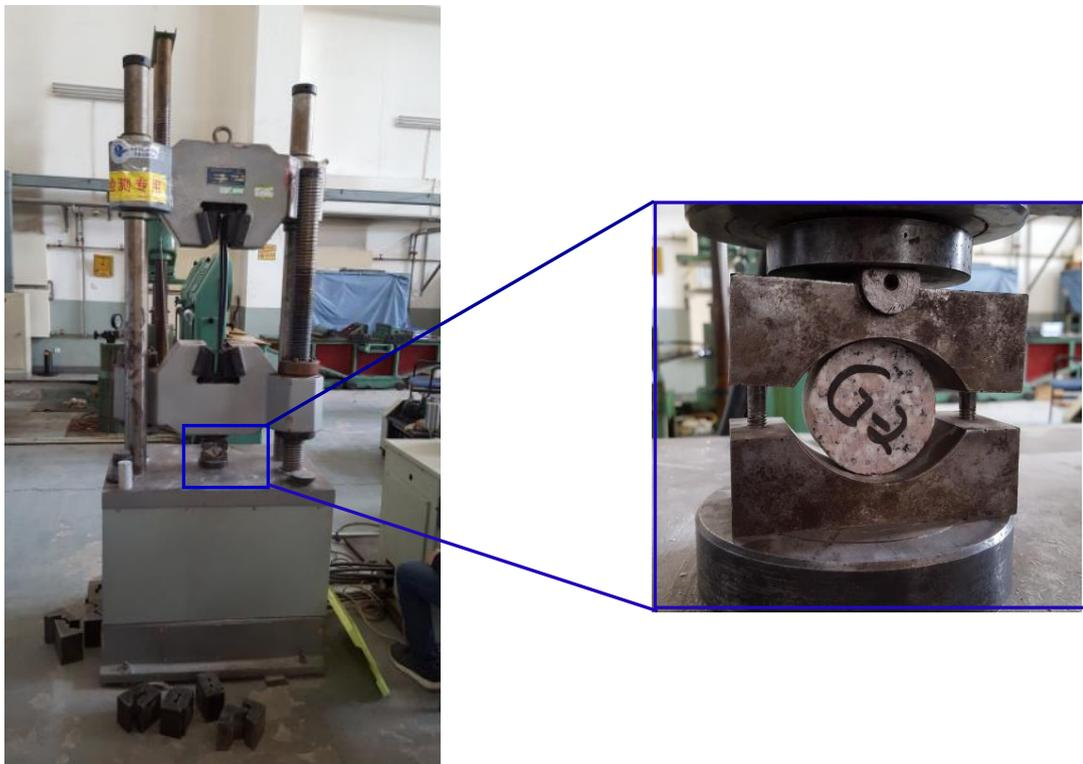
*Fig.2 - Hydraulic testing machine for Brazilian test*
