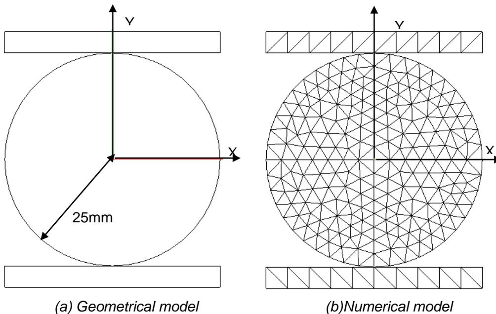
Fig.4 - Geometrical and Numerical model for BTS test
