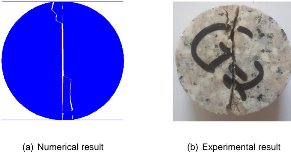
*Fig.7 - Comparison of the numerical and experiential results*
