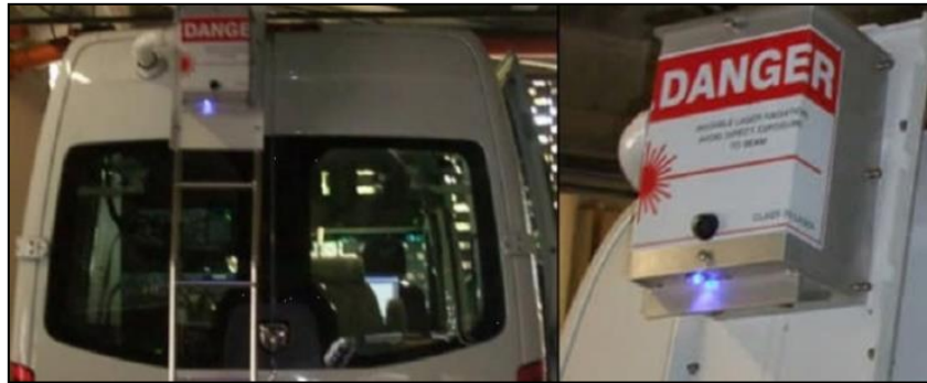
Figure 1 - A line-scan camera-laser illuminator device on a pavement survey vehicle
