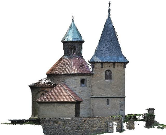
Figure 3 – Holubice – Photogrammetry derived point cloud section, North view
