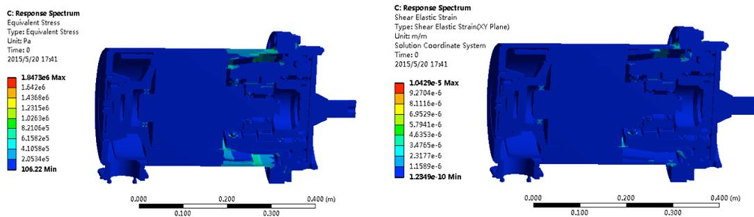
*Figure 5 - Integral Earthquake Response Spectrum Stress*
