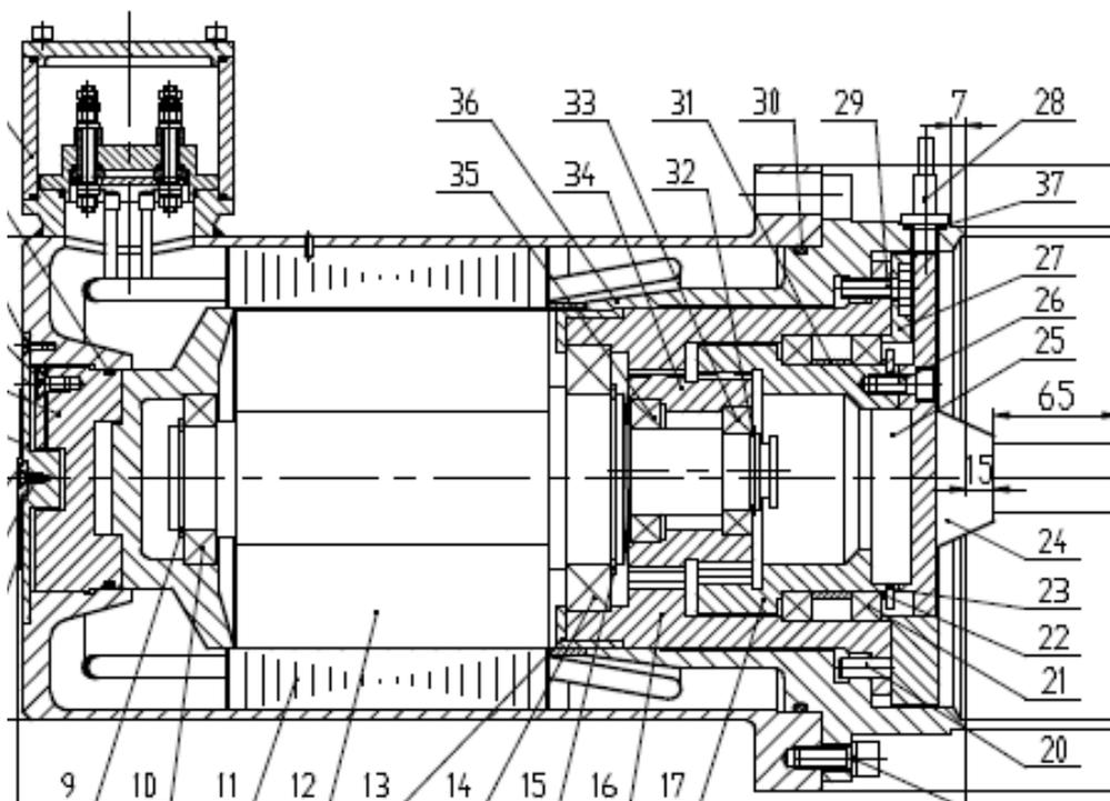
Figure 1 - Canned Motor Pump Drive Assembly Structure
