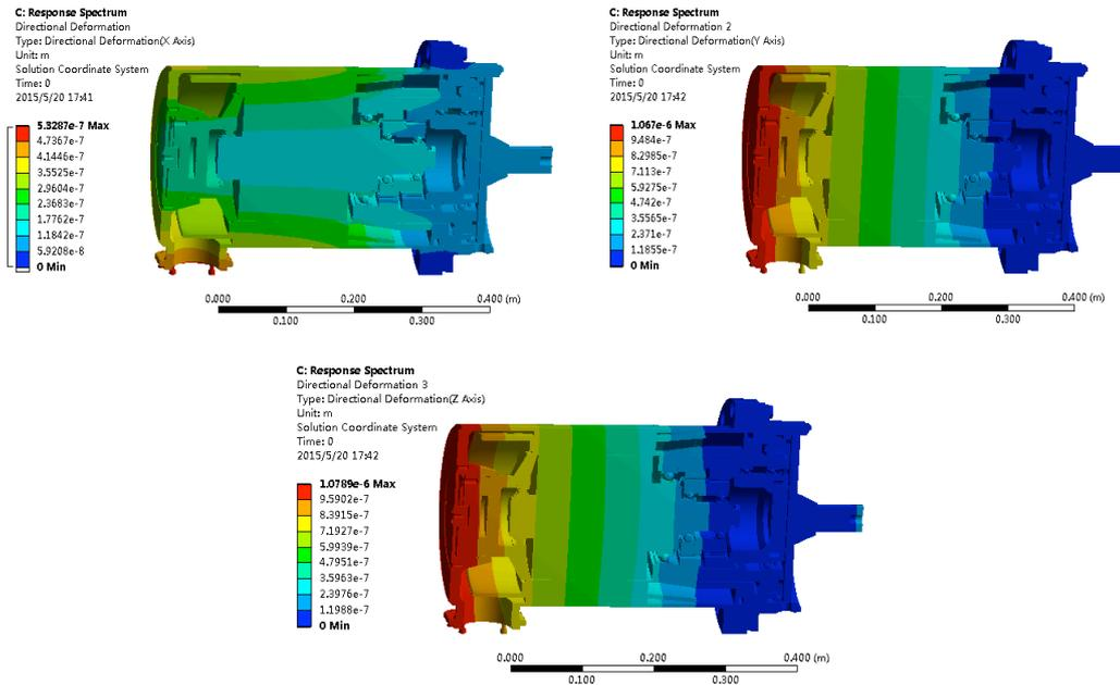
Figure 6 - Integral Earthquake Response Spectrum Deformation
