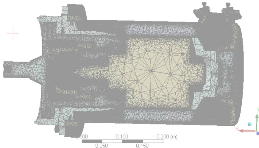
Figure 2 - Finite Element Mesh Model
