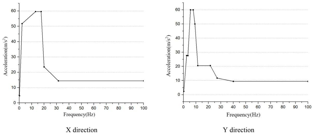
*Figure 4 - Earthquake Response Spectrum Input Curve*
