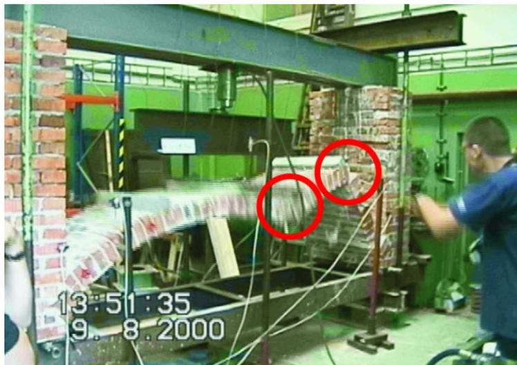
Fig. 2. - Vault collapse due to the supporting system's failure (horizontal displacement of supports)
