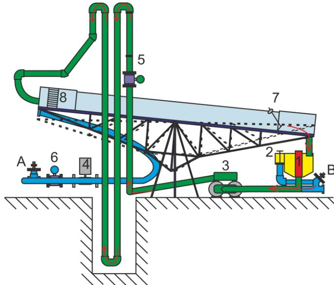
Fig 2: Tilting flume – 1 - supply and separation tank, 2 – overflow, 3 - centrifugal pump for mixture, 4 - centrifugal pump for water, 5 - flow meter for mixture, 6 - flow meter for water, 7 - outlet with overshoot weir, 8 - inlet with flow distributors, A, B - control valves
