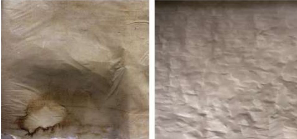
Fig. 2: a) Paraloid B72 nanotextile doped with TiO 2 , b) Paraloid B72 doped with Ag
