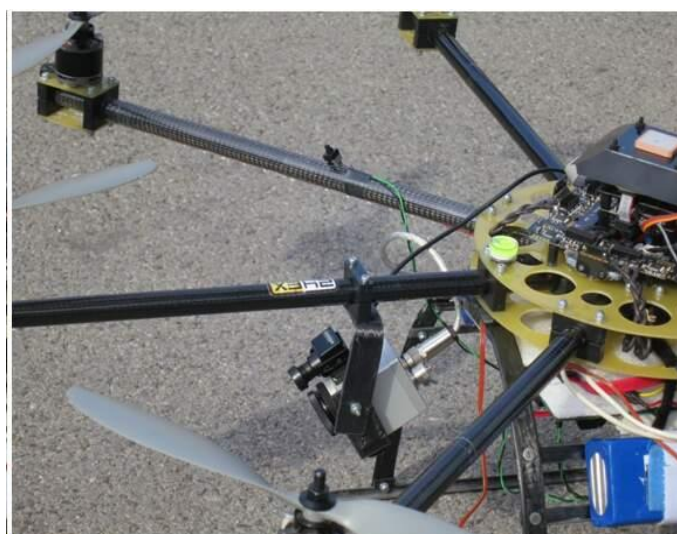
Fig. 4: Detailed view of thermal camera Optris and small surveillance camera
