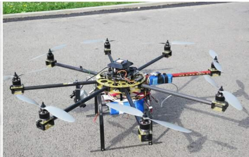
Fig. 3: Octocopter, load capacity to 1.5kg
