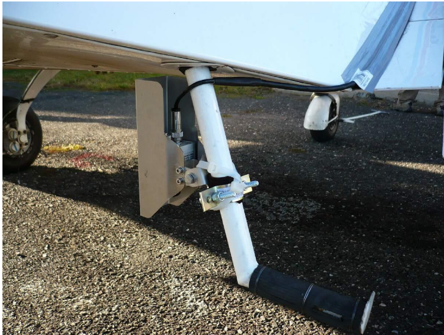
Fig. 9: Thermal camera Optris mounted on small aircraft
