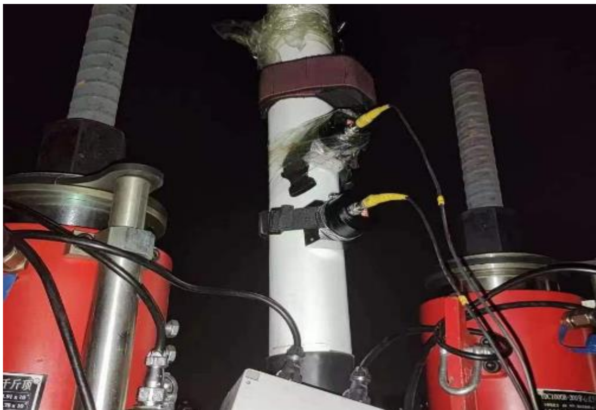
Fig. 6 – Cable force measurement
