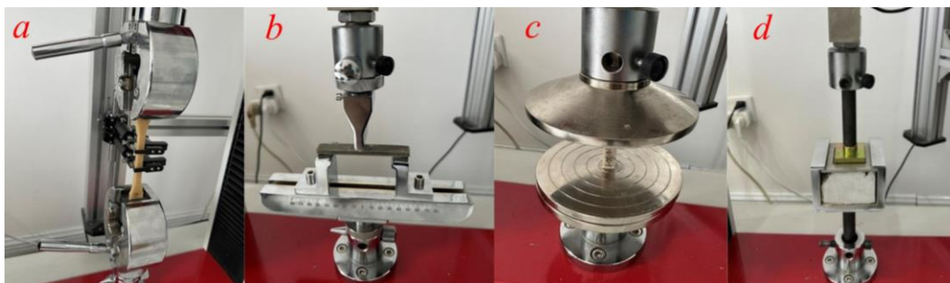
(a) Tensile test, (b) Flexural test, (c) Compressive test, (d) Test of normal tensile bond strength with concrete.
