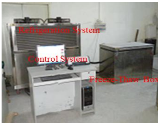
Fig. 2 – Freeze-thaw cycling system
