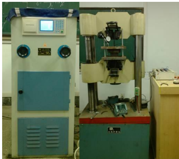
Fig. 11 – Pull-out test loading and data acquisition system
