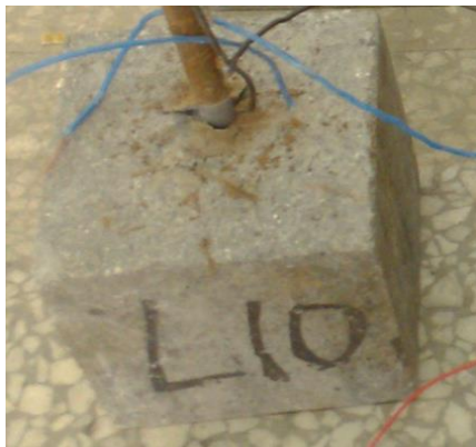
Fig. 14 – Failure mode of specimen L10
