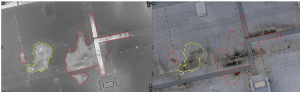
*Fig. 2 – Flat roof leak sample*
