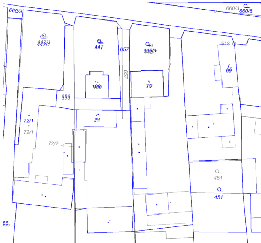
Fig. 8 – c. u. Vinice v Podkrkonoší – positionally correct property boundaries in KMD
