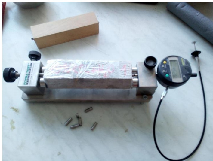
Fig. 3. – FORM+TEST strain gauge.
