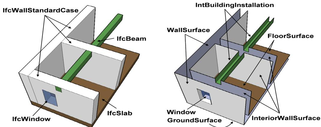
Figure 5: Differences between geometry representations in BIM and 3D GIS [23]
