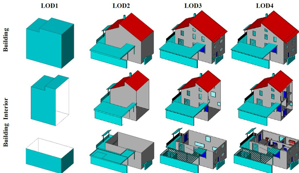
Figure 3: A building model in CityGML LOD1 – LOD4 [7]
