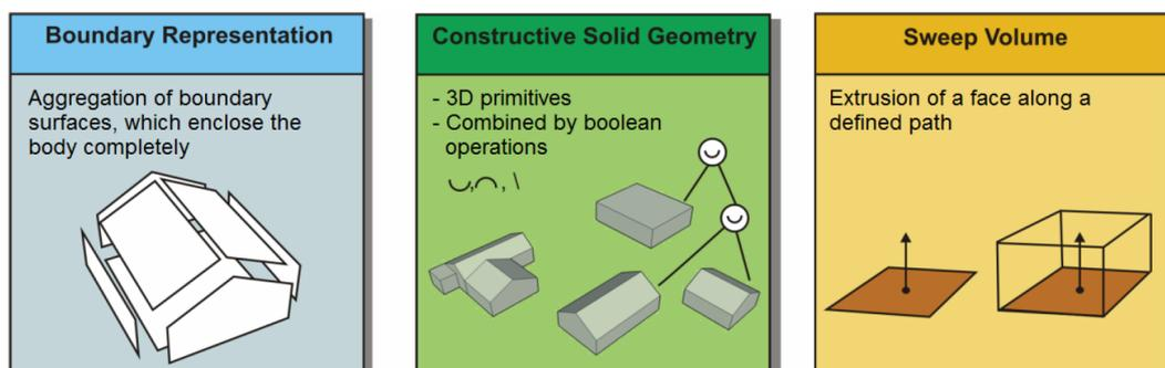
Figure 2: The ways of geometry representation in IFC [8]
