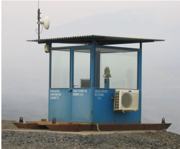
Figure 1: Total station in the protective shelter.
