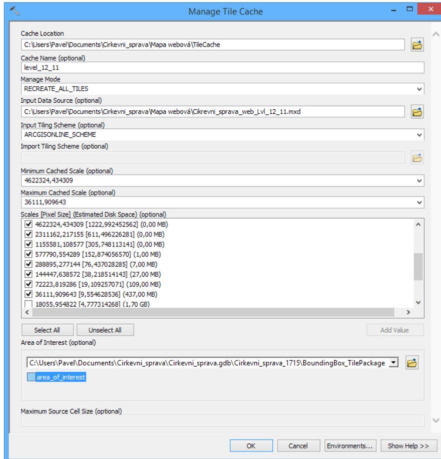
Figure 6: *Manage Tile Cache* tool settings which generates map tiles.
