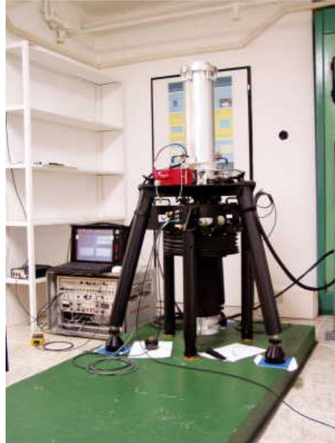
Figure 1: Absolute gravimeter FG5 n.215, Geodetic observatory Pecný.
